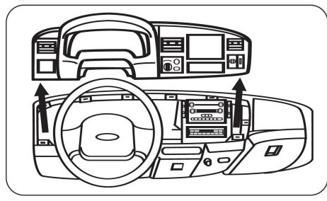
3 Remove (4) 9/32" screws to remove the factory radio. (Figure B)
