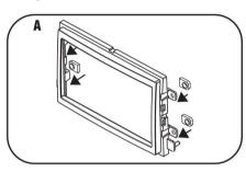
3 Attach the double DIN brackets to the radio housing. **Note:** The notch in the housing should be on top. (Figure 3A,3B)
